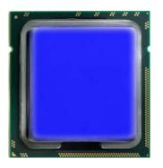
The surface highlighted in blue is part of the metal cap and is covering the quad or dual cores in picture QP1. If the metal cap does not have existing thermal material on it, cleaning is not required, but is highly recommended. If any existing thermal material is on the metal cap, the surface must be cleaned prior to applying your new thermal compound.
